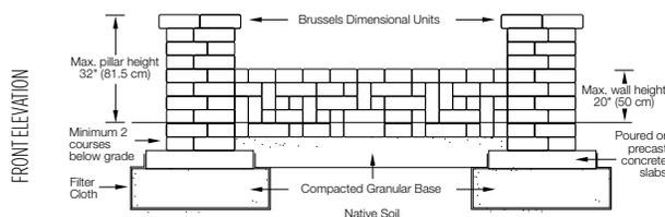
All joints must be adhered with Unilock approved Concrete Adhesive. Base preparation may vary according to soil and climate conditions. Cross sections are examples, and must not be used for construction.
