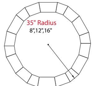
Although the three tapered unit sizes come packaged together, they can be separated to achieve various radius projects. If you construct a radius using only one size unit, the other units will be left over. Careful planning will allow you to use these units elsewhere.
