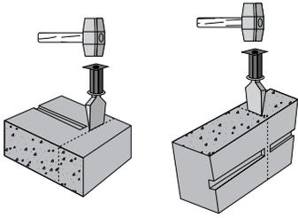
To split a large convertible unit, use a hammer and chisel to score the top and sides, then flip the unit upside down and use the chisel to break the unit. This may require a couple of hits along the groove to achieve a clean break.
