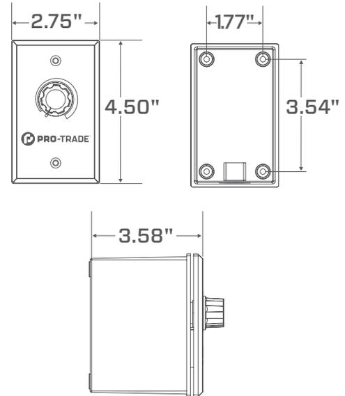
12V LED lamp dimming performance will vary. Trim dial adjustment will be needed depending on wattage load and number of lamps on the circuit. The Pro-Trade® LED dimmer is intended for use with magnetic 12VAC landscape transformers and 12VAC lamps only. Do not exceed the maximum wattage or load capacity listed above.
